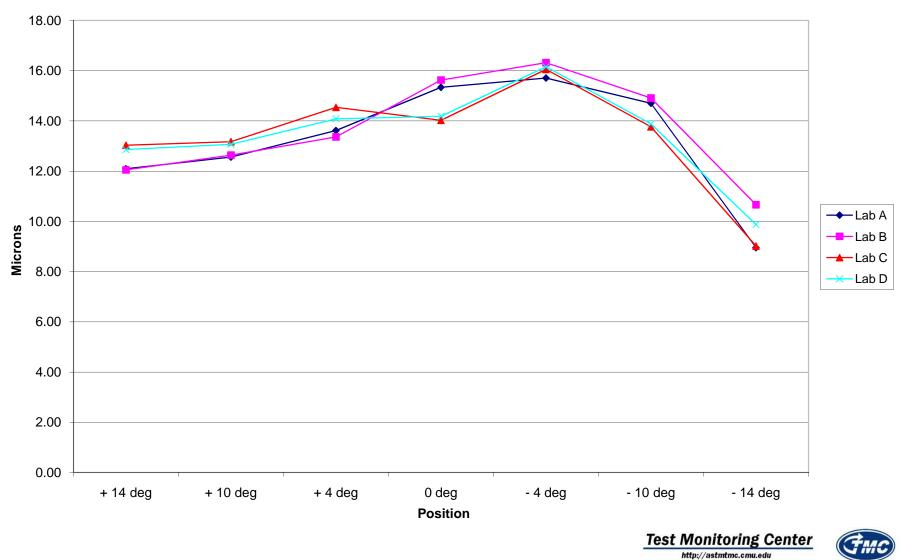
Sequence IVA Round Robin Camshaft Wear Profiles, Max Intake
