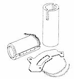
To increase the heating efficiency of your application, silicone rubber heaters can be thermally insulated with silicone sponge rubber, bonded to one side in the following thicknesses:  $\chi_6$ ,  $\chi$ ,  $\chi$ ,  $\chi$  or  $\chi$  in. (1.6, 3.2, 6, 9.5 or 13 mm). Heaters with thermal insulation are still quite flexible.
