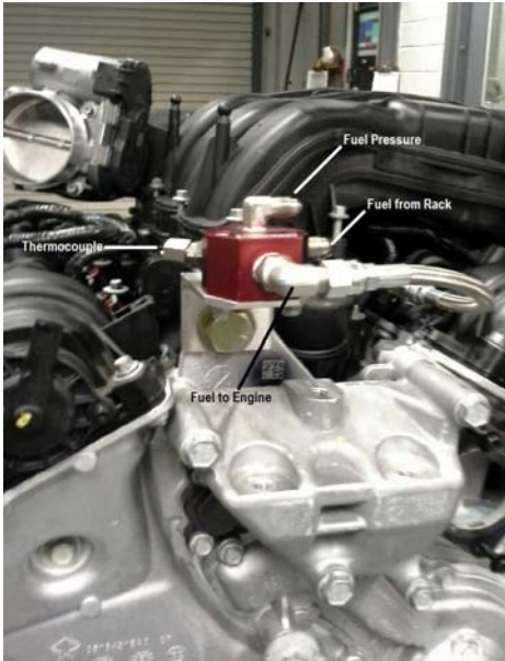
FIG. A2.4 to A2.5 Fuel Temperature, Pressure and Supply
