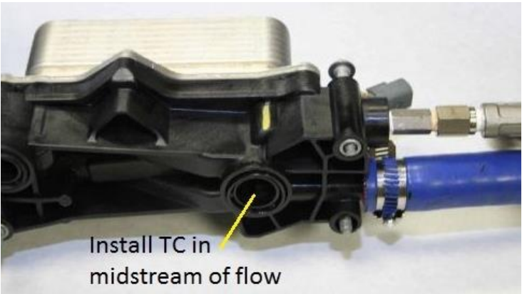
FIG. A2.6 to A2.7 Oil Cooler Temperature and Oil Gallery Pressure
