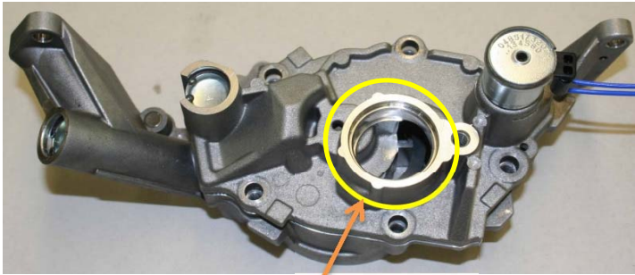
Pickup Tube, Suction Side of Pump
