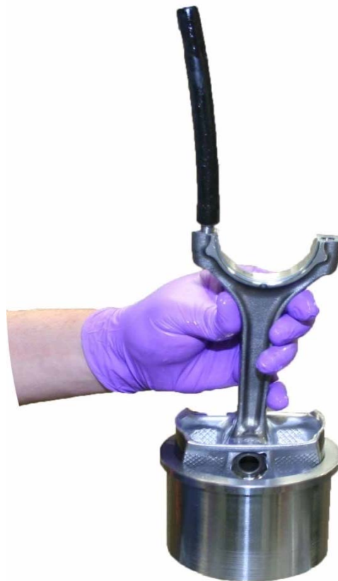
Piston ring installation sleeve with rubber tubing used as an installation guide (In-house fabricated)
