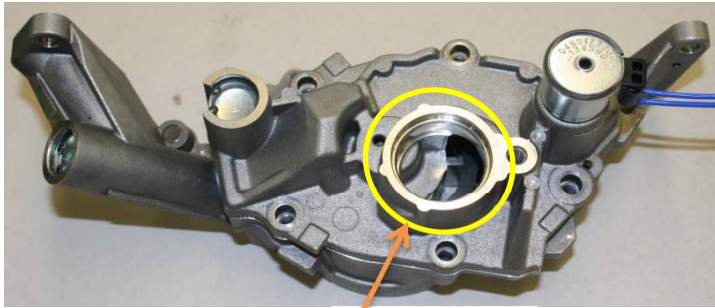
Pickup Tube, Suction Side of Pump
