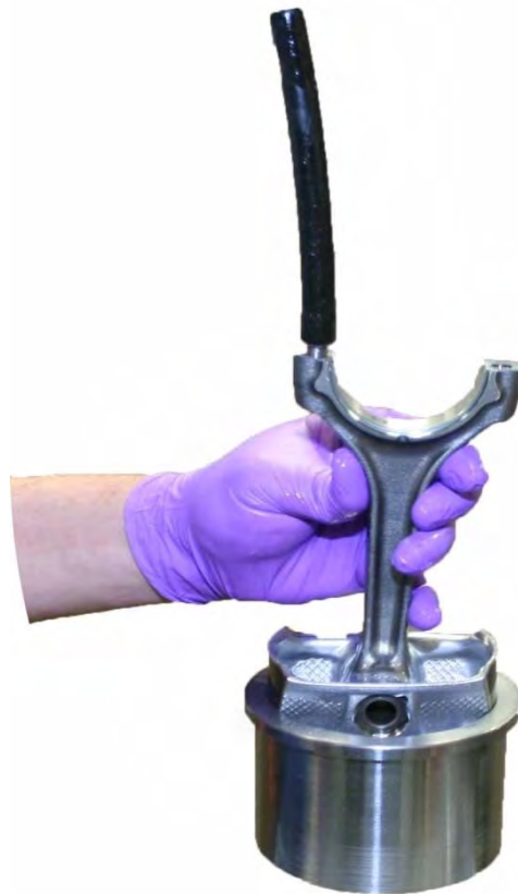
Piston ring installation sleeve with rubber tubing installation guide (In-house fabricated)
