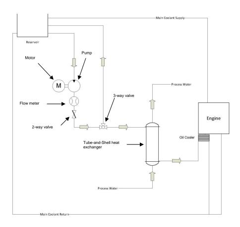
Fig. A15.1 Typical Engine Oil Cooling System Schematic
