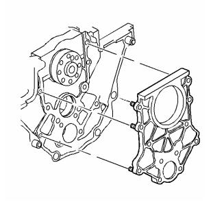
4. Install the crankshaft rear oil seal housing housing onto the engine. Make sure to use a new oil seal housing gasket.
