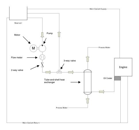
Fig.A15.1 Typical Engine Oil Cooling System Schematic
