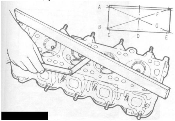
Using a straight edge, measure the clearance between the straight edge and the head with a feeler gauge. Maximum .004"
