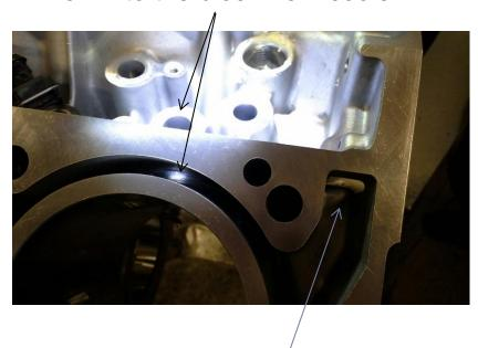
Flow into the block from pump
