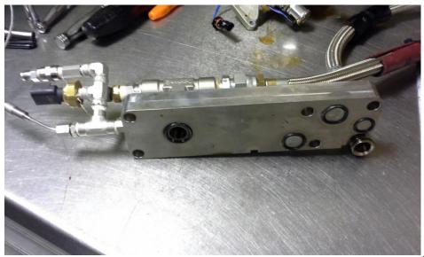
We originally ran with this plate in place of the oil cooler. Eleven tests were run with the oil being conditioned outside the engine.
