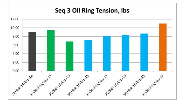
Tension measured at 3.800" diameter
