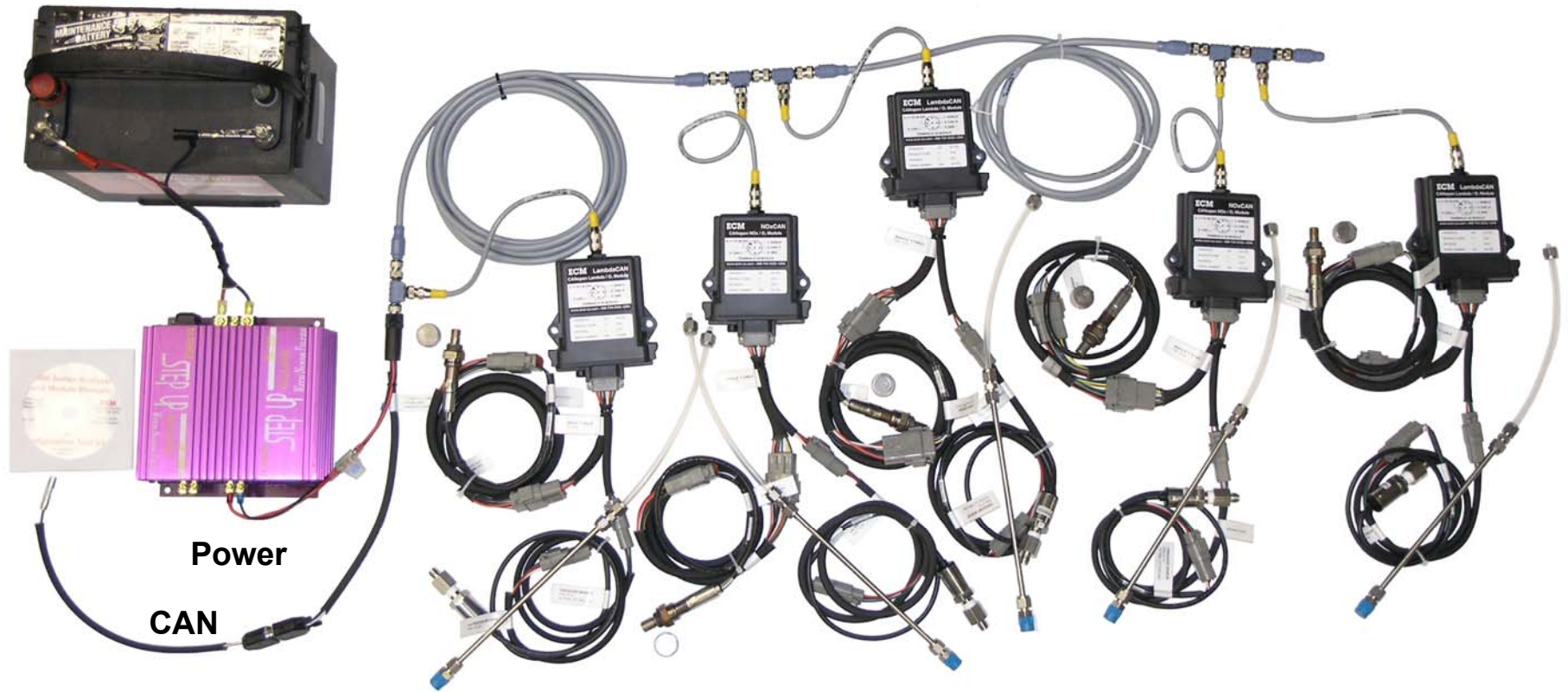
Example: 5 Channel (3 LambdaCAN, 2 NOxCAN) Pressure Compensated System
