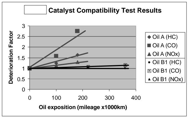
It is clear from the pictures that oil type B1 causes a much lower increase in emission compared to oil type A, even though the total amount of exposed oil is higher.
