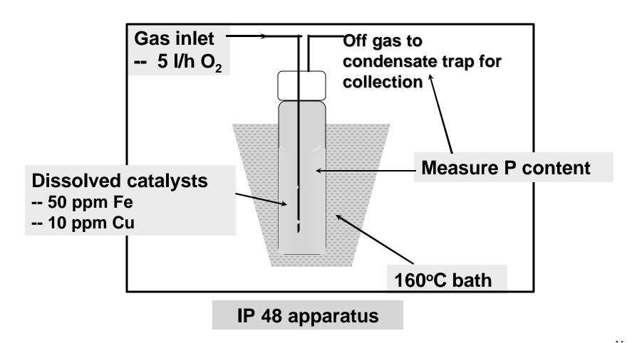
Bulk oil aging addresses the crankcase model
