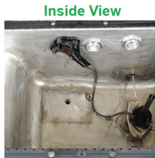
Fig. A5.6 Oil Sump Thermocouple Location
