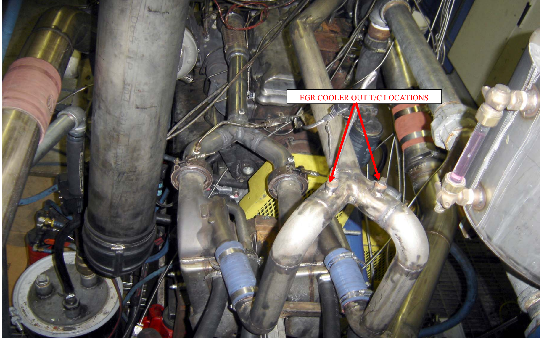
FIG. A1.14 EGR COOLER OUT TEMPERATURE
