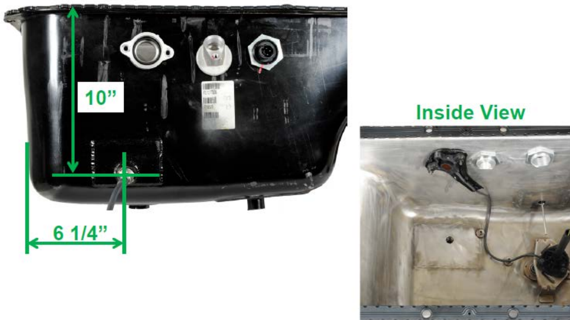
Oil Sump Thermocouple Location
