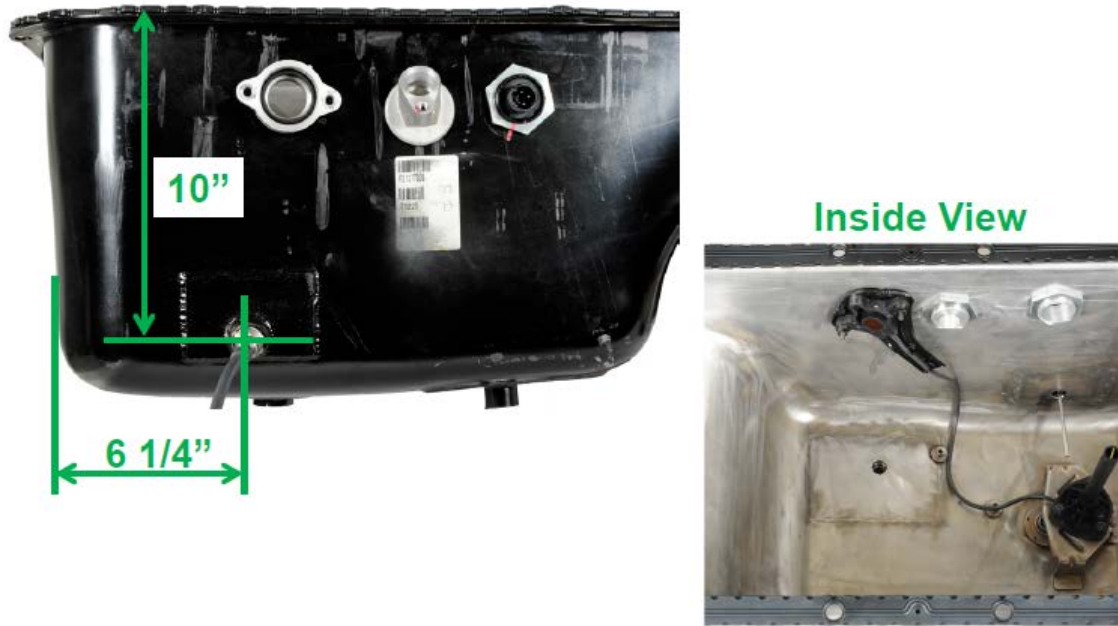
Oil Sump Thermocouple Location
