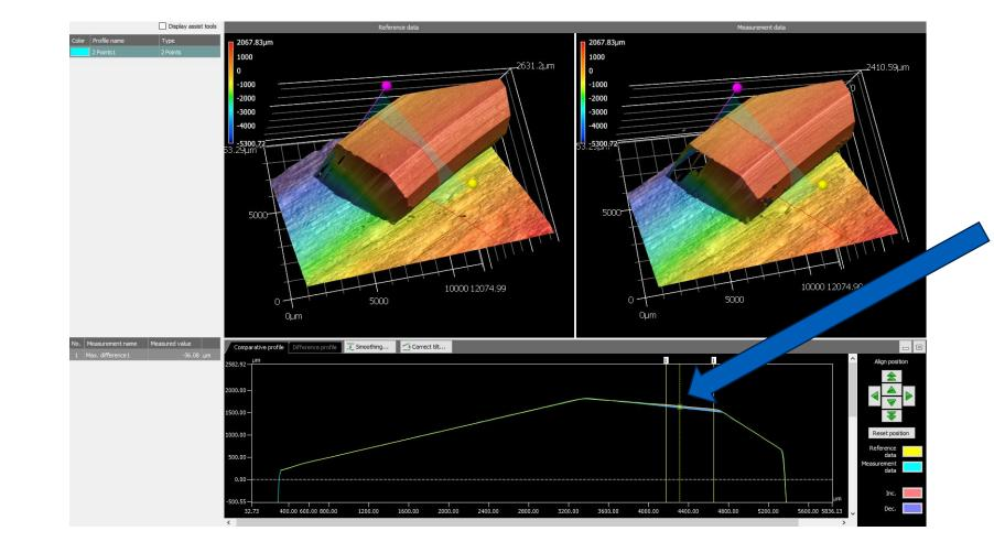
Max difference between profiles at any point -36.08 microns
