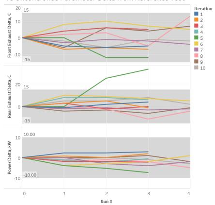
Both alternate fuel tests shall be operationally valid with no controlled parameters outside of prescribed average limits.
