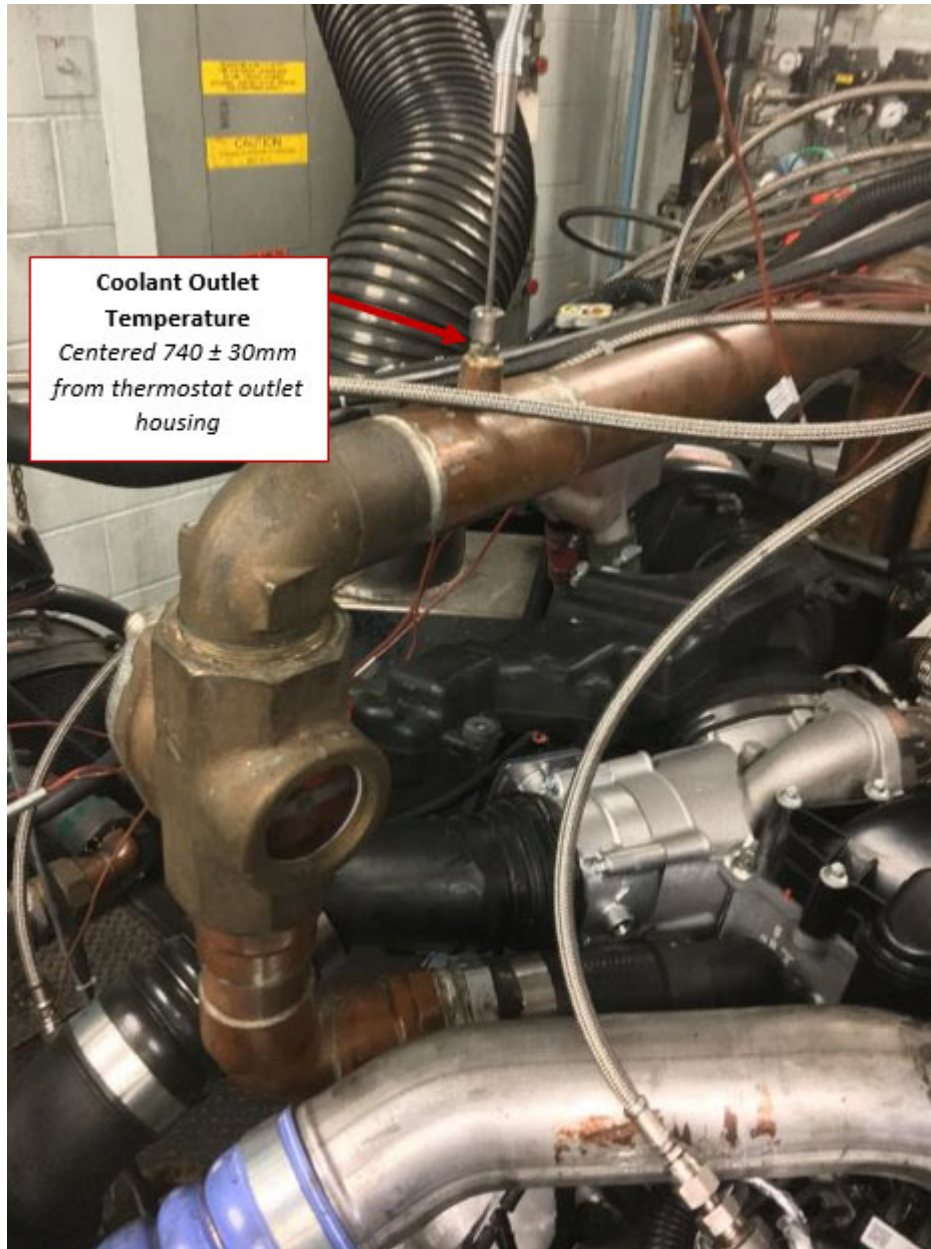
Figure A4.28 Engine Coolant-Outlet Thermocouple Location
