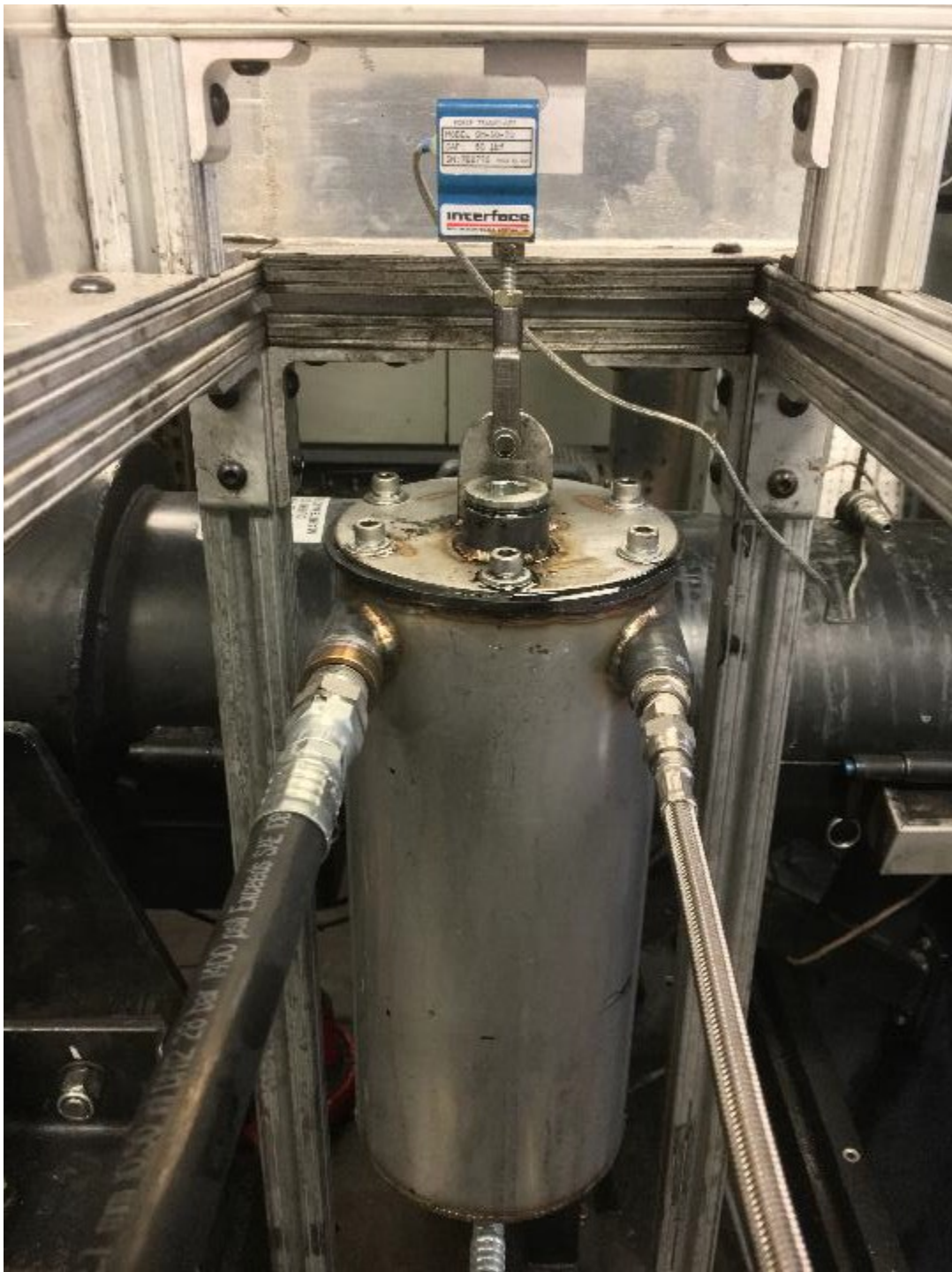
Figure A4-33 Example of Auxiliary Oil Reservoir Suspended from a Load Cell
