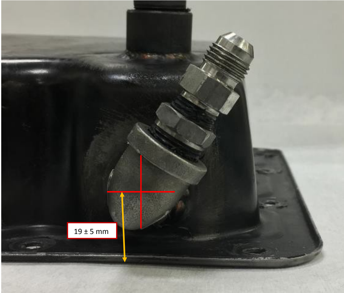
Figure A4-17 Auxiliary Oil System Return Port on Rear of Pan (Rear View)
