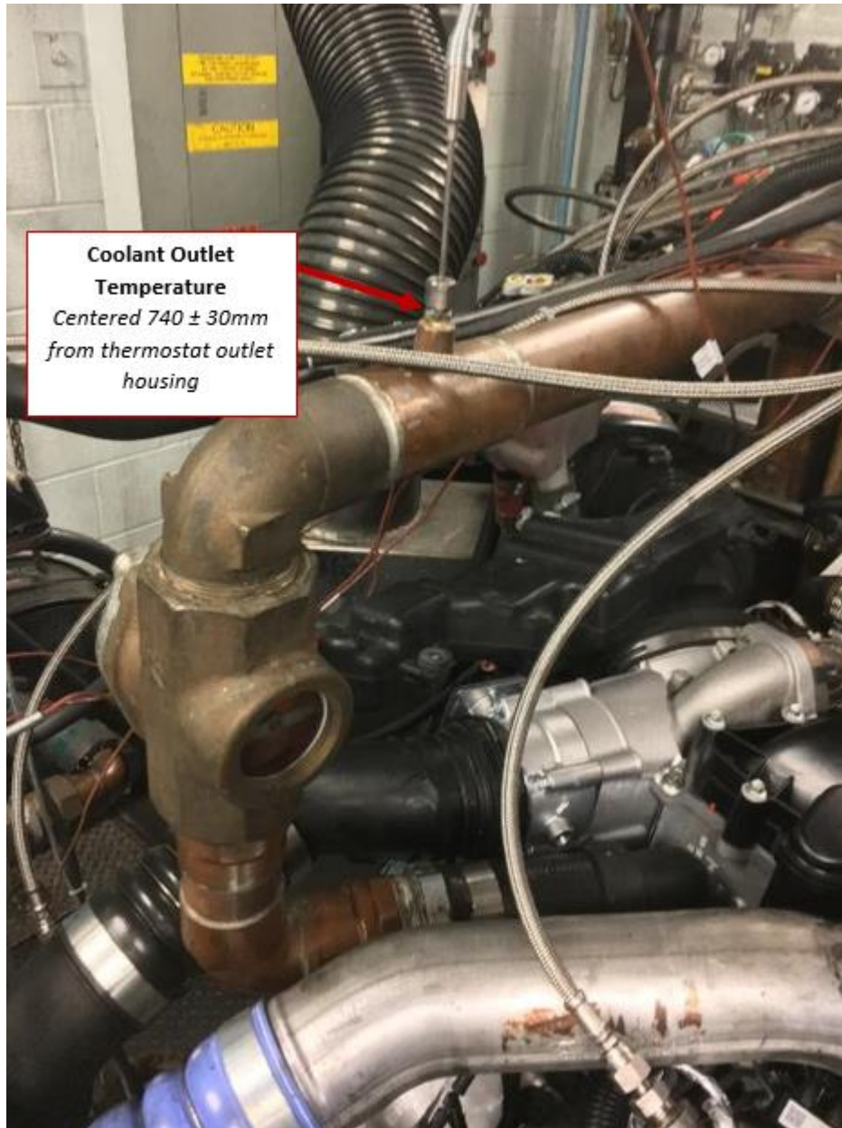
Figure A4.28 Engine Coolant-Outlet Thermocouple Location
