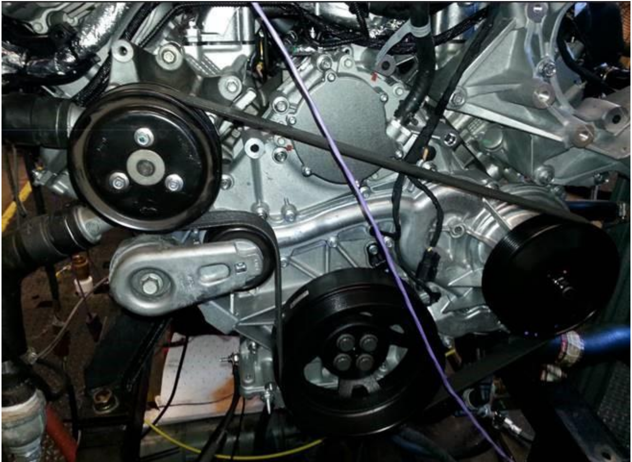
Figure A4.12 Front End Accessory Drive
