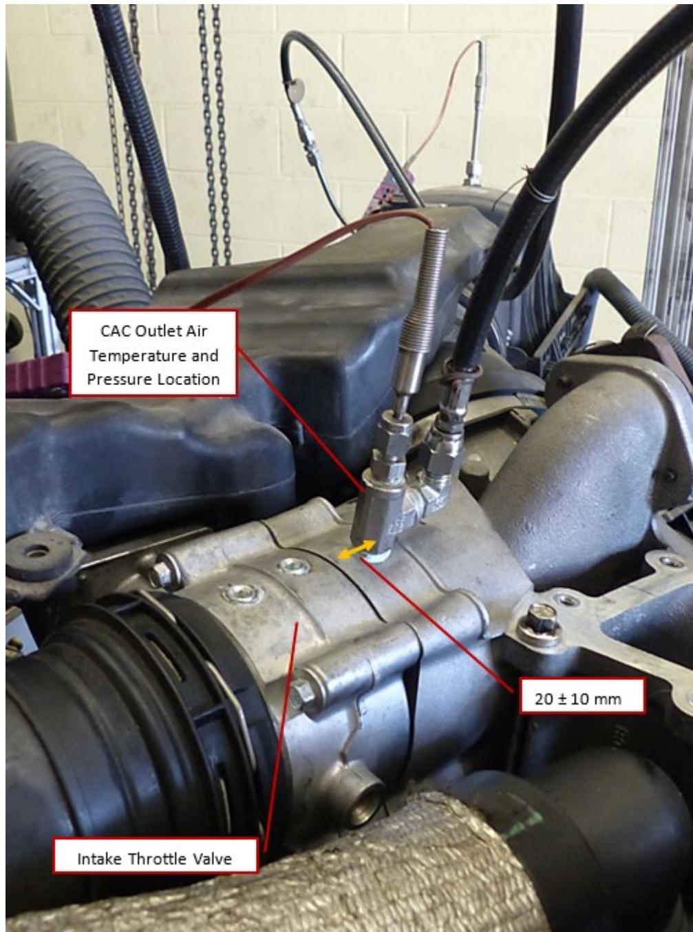
Figure A4.20 Air Temperature at CAC Outlet Thermocouple Location
