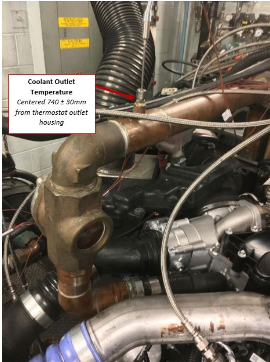
Figure A4.28 Engine Coolant-Outlet Thermocouple Location
