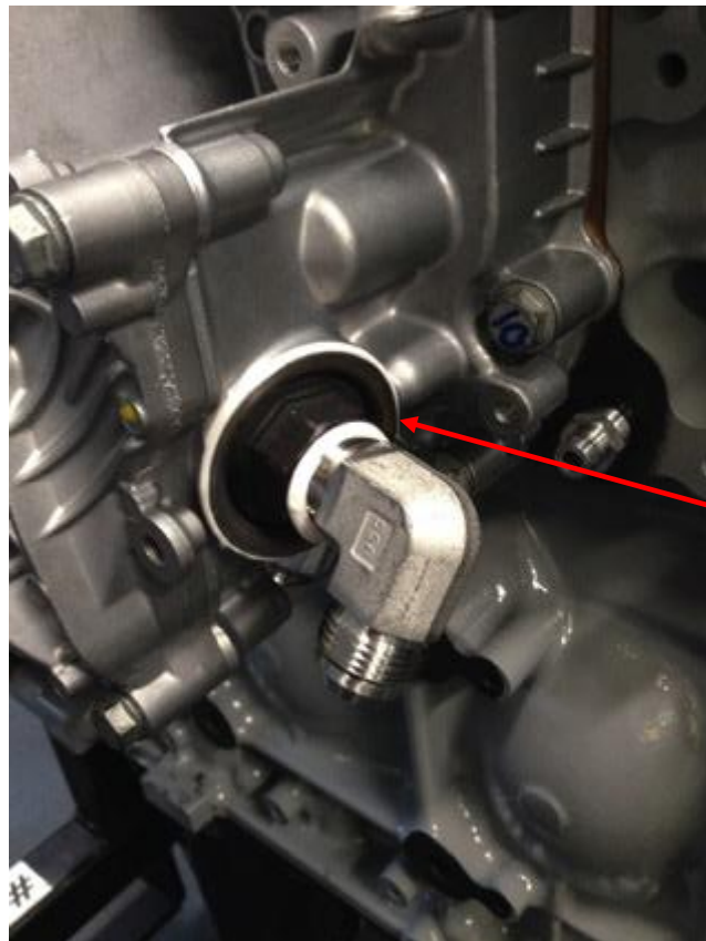
FIG. A4.10 Oil Module to Remote Oil Heat Exchanger Return Modification
