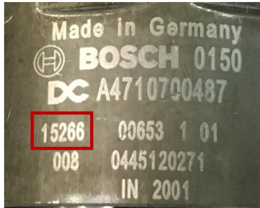
FIG. X1.1 Location of Date Codes for Injector Nozzles
