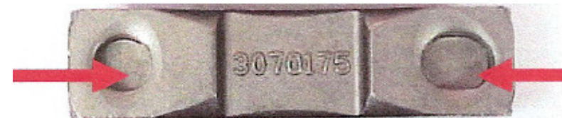
Effective case depth measured in pockets
