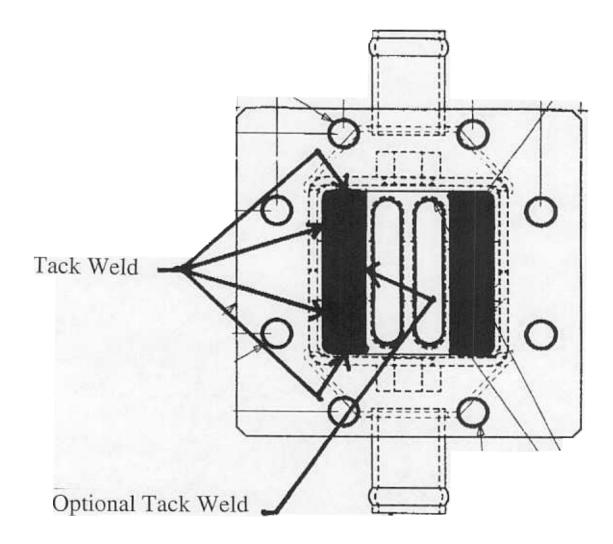
.06 inch Stainless Steel Plate Fit Into Recess
