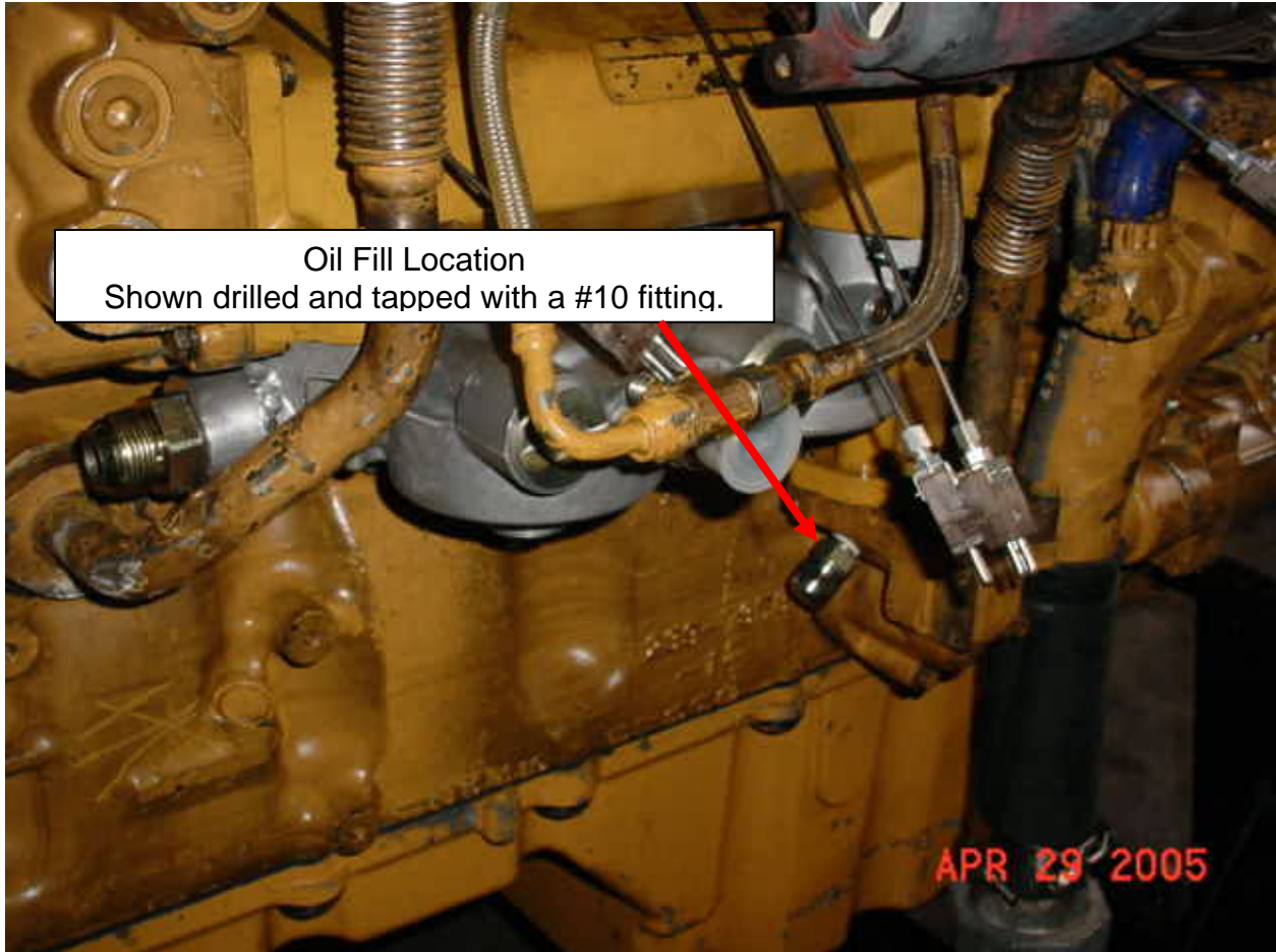
Fig. A4.21 Pressurized Oil Fill Location
