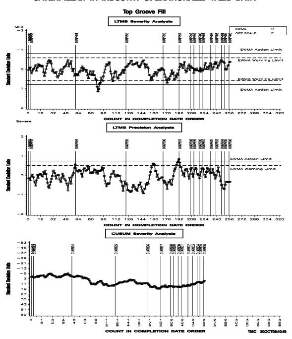
The LTMS/Cusum plot for TGF is shown above. TGF severity and precision remained within limits this period.
