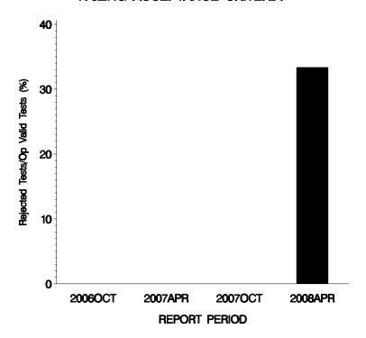
One test failed this period for severe WDN. Another test failed in the April 2006 report period (also severe WDN). Those two tests are the only 1N tests to fail since August of 2001.
