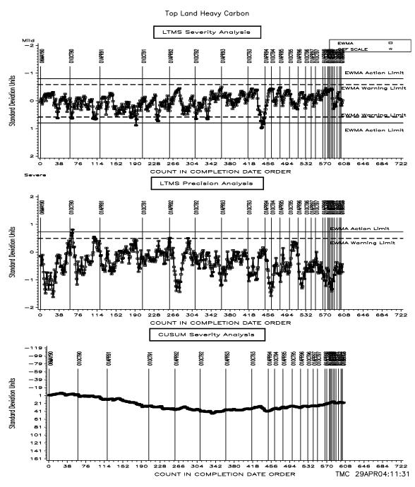
The LTMS/Cusum plot for transformed TLHC is shown above. Precision and severity were both within limits throughout this report period.
