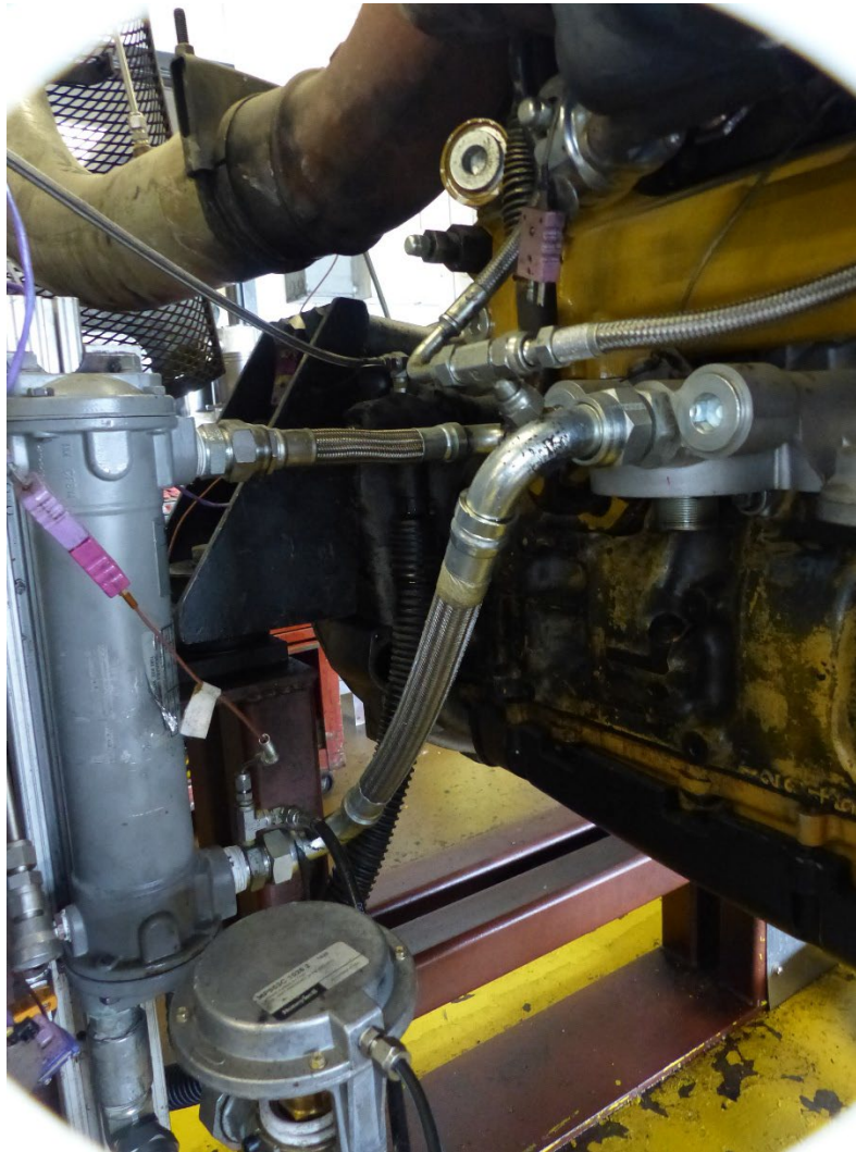
FIG. A5.15 External Oil Heat Exchanger Outlet Pressure
