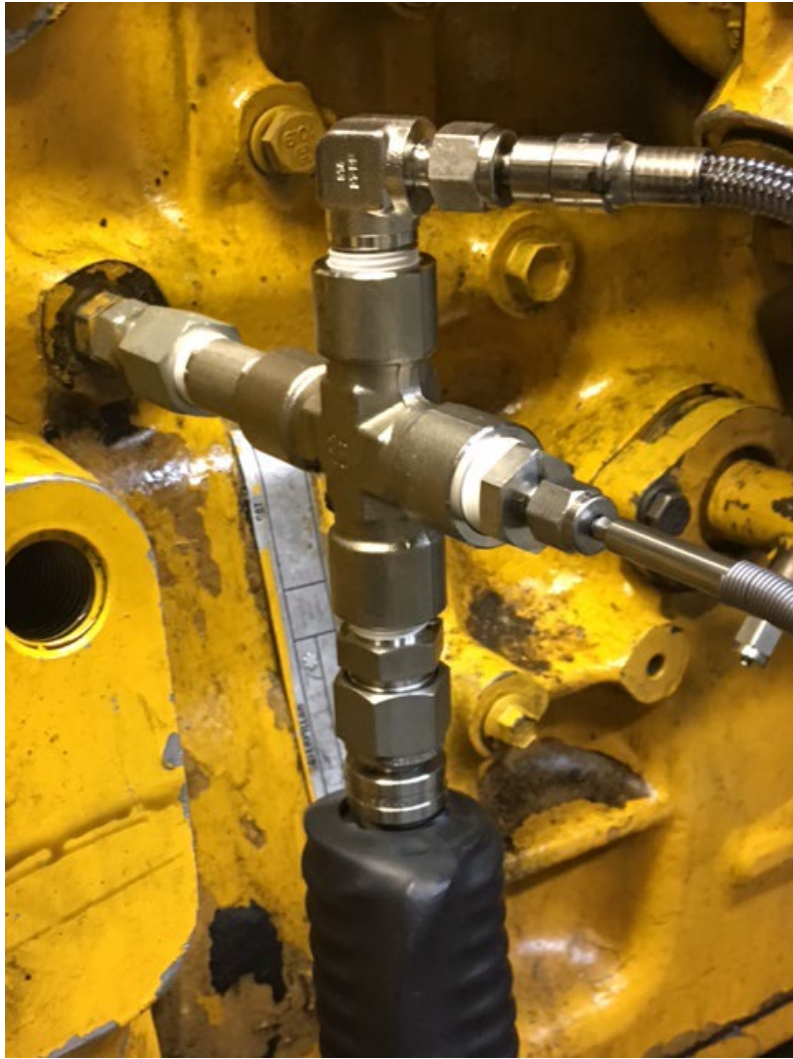
FIG. A5.11 Oil Gallery Sample Fitting with Heated Line, Pressure and Temperature Measurements
