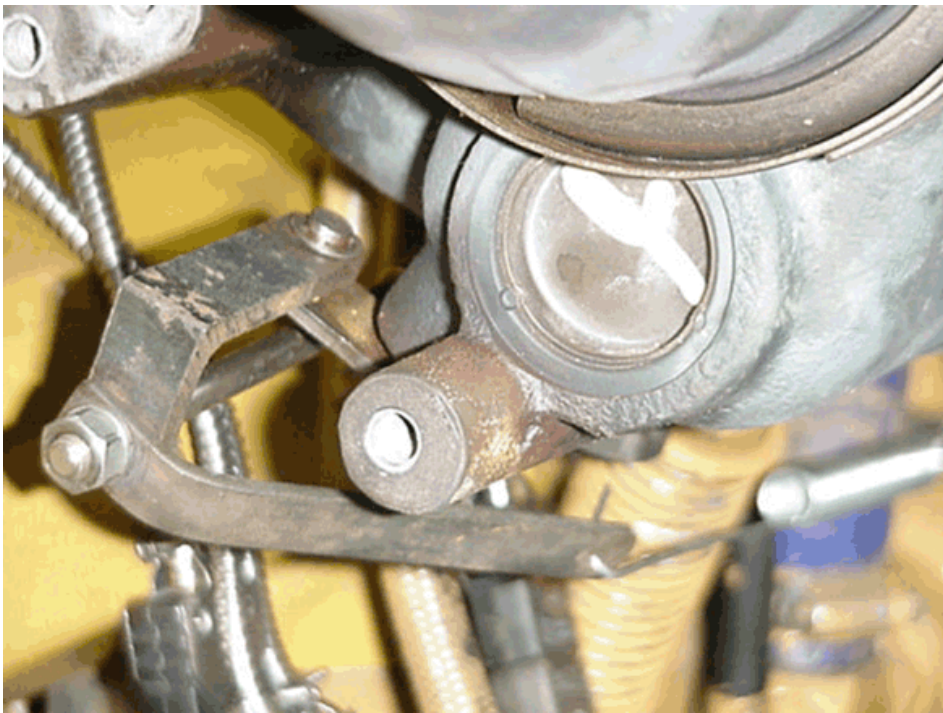
FIG. A5.21 Turbo-Waste-gate Control
