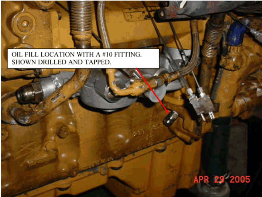
FIG. A5.24 Location for Pressurized Oil Fill
