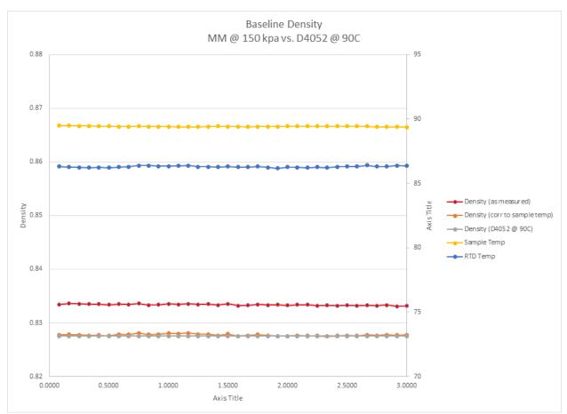
McCord showed a graph (below) of warm up data (150kpa sample pressure and ~90C sample temp) with density corrected to the sample temperature.
