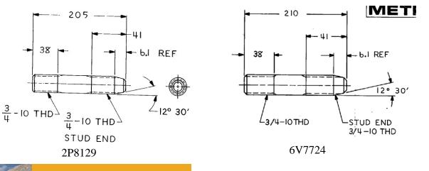
5 mm longer Washer can be added under the nut Or one of the ends machine-turned shorter
