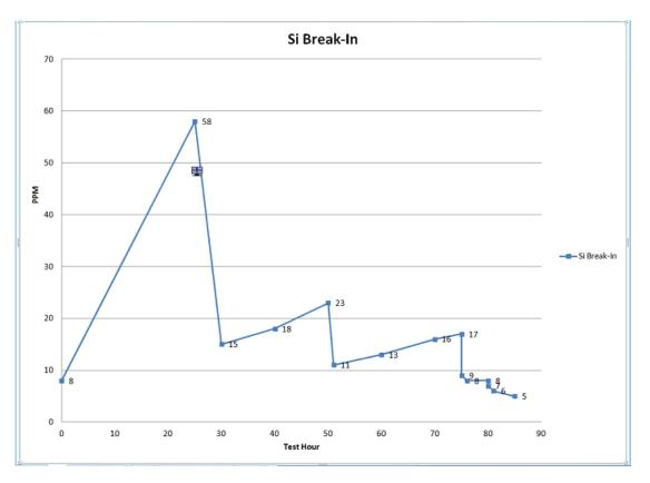
Action: Agreement that the SWRI engine is broken in and then will proceed to the shakedown testing using the LZ oil.
