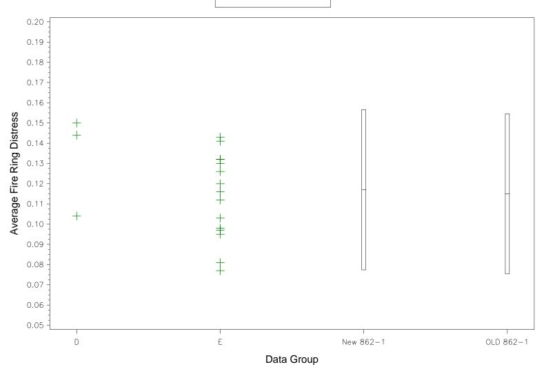
6V92: Reference Oil 862-1 Test Target Data Set and Shewart Severity Limits
