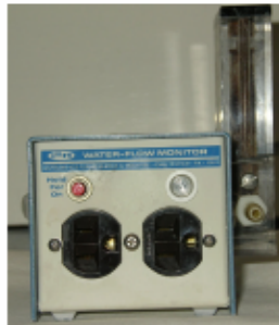
Water Flow Monitor
