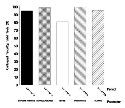
The above chart shows the percentage of accepted operationally valid tests. This period one silicone test, one ethylene acrylate test, and four nitrile tests failed to meet the acceptance criteria.
