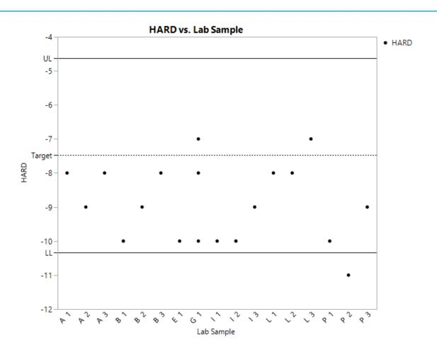
Most of the SL107 HARD are below the target and Lab P, Sample 2 is outside the 3 s limits.
