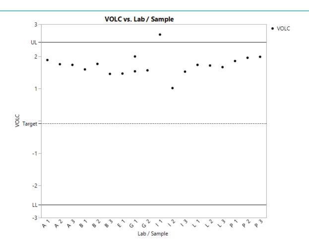
All VOLC are above the target and Lab I, Sample1 exceeds the 3 s limits.
