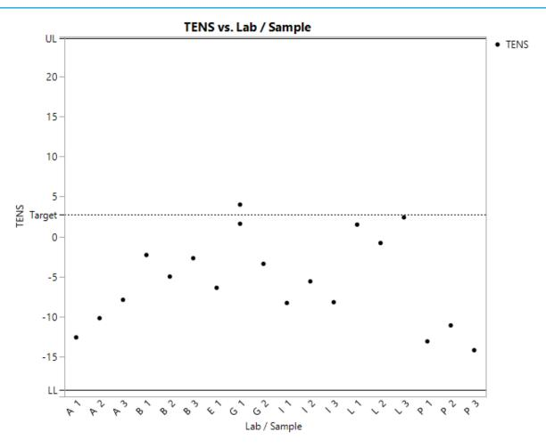
All SL107 TENS are within the 3 s limits though all but 1 are below the target.
