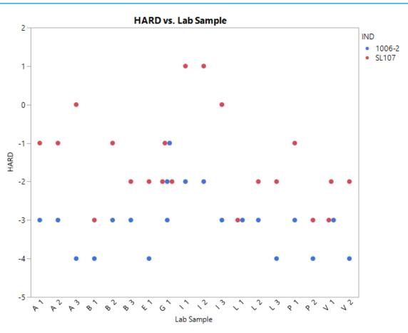
For each bath pair, HARD for SL107 is equivalent or higher than 1006 2.
