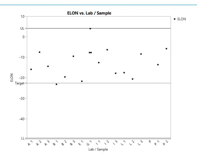
All SL107 ELON are within the 3 s limits though only 1 is below the target.
