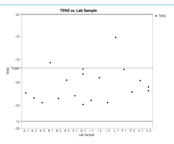
All SL107 TENS results are within the 3 s limits though all but 2 are below target.
