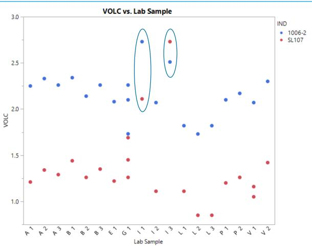
Lab I, Samples 1 and 3 are outside the range of the other samples for both oils.
