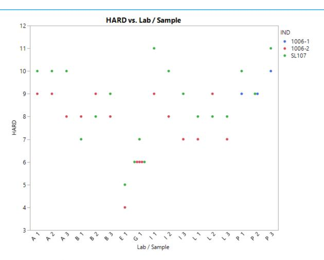
For most pairs, SL107 is a unit higher in HARD relative to 1006.
