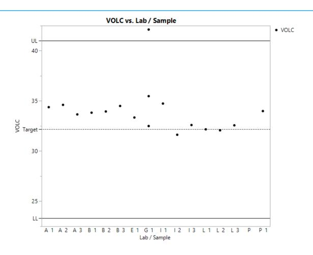
Most of the VOLC are above the target and 1 of the Lab G results exceeds the 3 s limits.
