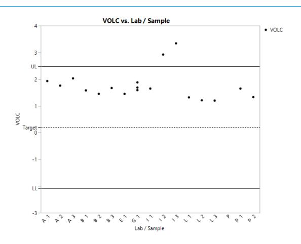
All VOLC are above the target and Lab I, Samples 2 and 3 exceed the 3 s limits.
