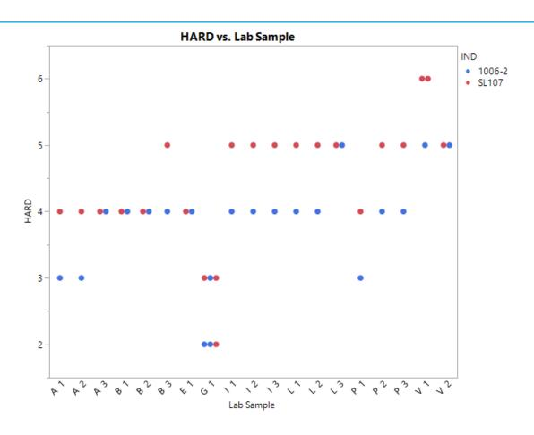
For each bath pair, the HARD for SL107 is equal to or a unit higher than 1006-2.
