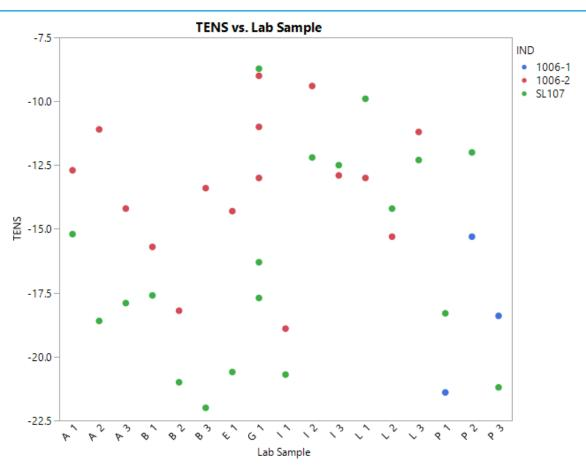
The Reference Oil correlating to the higher (less negative) TENS is mixed amongst the pairs indicating similarity in Reference Oil means.
