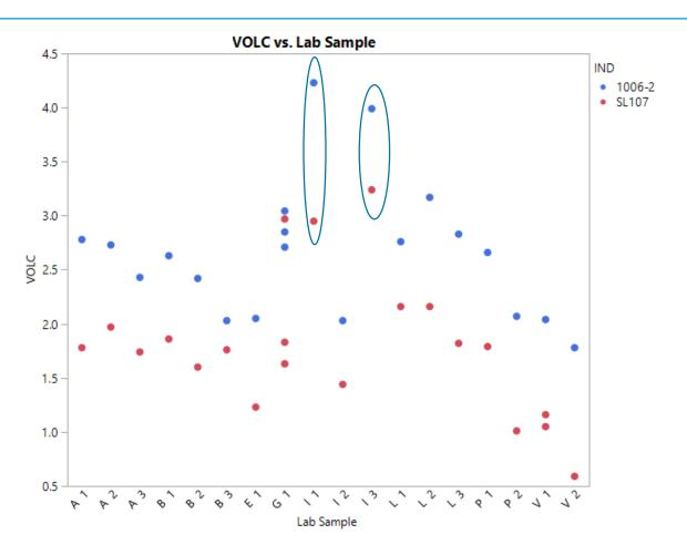
Lab I, Samples 1 and 3 are outside the range of the other samples for both oils.
