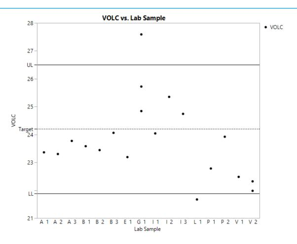
• 2 SL107 VOLC results (1 of Lab G, Sample 1 and Lab L, Sample 1) exceed the 3 s limits.
