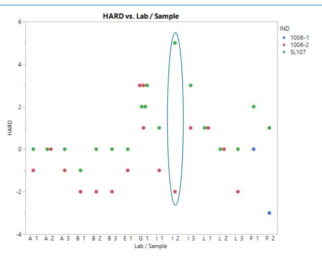
The difference between SL107 and 1006 for Lab I, Sample 2, is higher than for other bath pairs.
