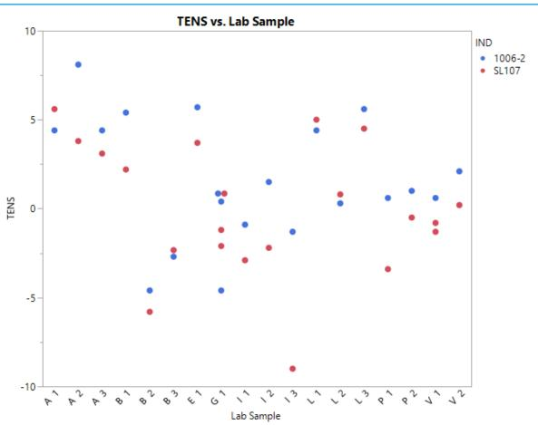
The Reference Oil correlating to the higher (less negative) TENS is mixed amongst the pairs indicating similarity in Reference Oil means.
