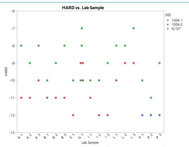
For each bath pair, the Hardness for SL107 is higher (less negative) than 1006.
