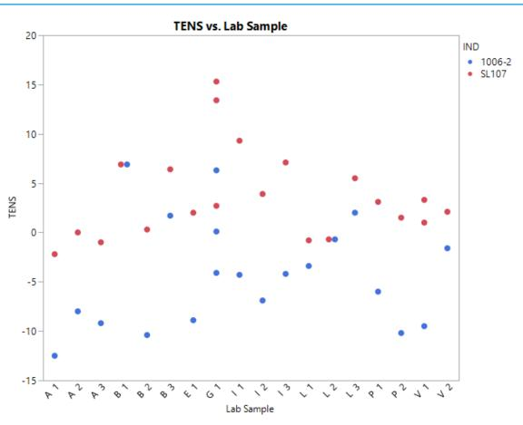
For each bath pair, TENS is equal to or higher (less negative) for SL107 relative to 1006-2.
