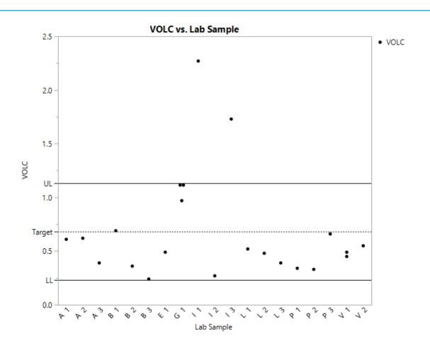
• 2 SL107 VOLC results (Lab L, Samples 1 and 3) exceed the 3 s limits and 4 others are just within the limits.
