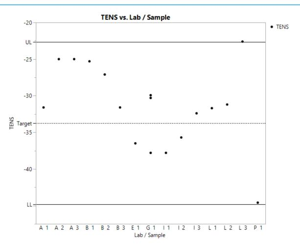
1 (Lab L, Sample 3) SL107 TENS exceeds the upper 3 s limit and 1 (Lab P, Sample 1) is just above the lower 3 limit.
