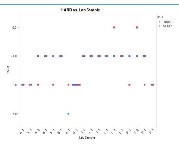
For each bath pair, HARD for the 2 oils is no more than a unit different.
