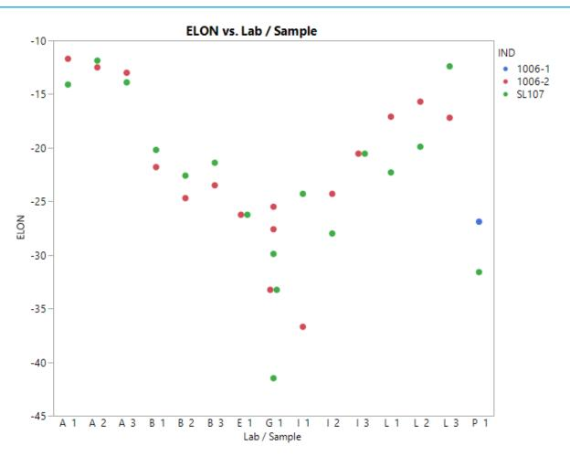
The Reference Oil correlating to the higher (less negative) ELON is mixed amongst the pairs indicating similarity of means.
