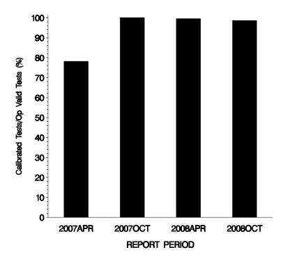
The above chart shows the percentage of accepted operationally valid tests. The April, 2007 period shows less than 100% because of the 128 operationally valid tests that were used to generate data on a new filter paper batch but were not used for calibration.
