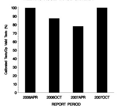
The above chart shows the percentage of accepted operationally valid tests. Last period shows less than 100% because of the 128 operationally valid tests that were used to generate data on a new filter paper batch but did not count towards calibration.
