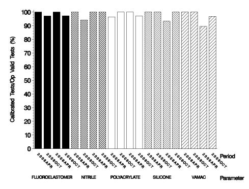
The above chart shows the percentage of accepted operationally valid tests. This period one fluoroelastomer test, on polyacrylate test, and one vamac test failed to meet the acceptance criteria.
