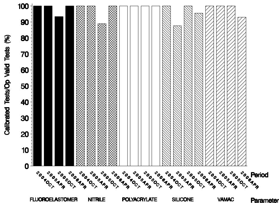
The above chart shows the percentage of accepted operationally valid tests. This period one silicone and one VAMAC tests failed to meet the acceptance criteria.
